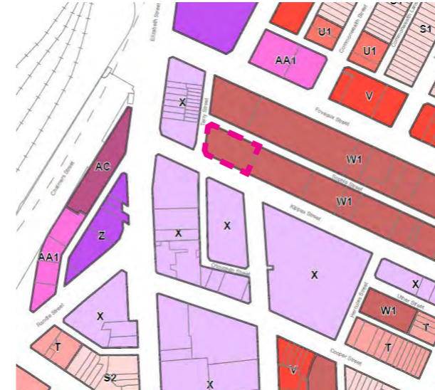
FSR: Floor Space Ratio W1 = 3.5
